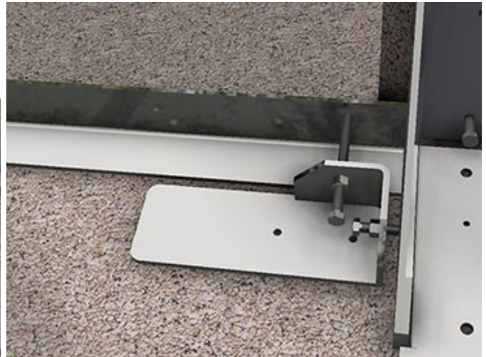
Temporary adjustment blocks used for positioning the Fixing Frame
