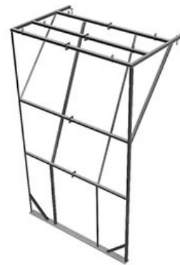
The temporary Measuring Frame, fixed to the Fixing Frame
