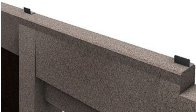
Reference brackets fixed to existing concrete structure
